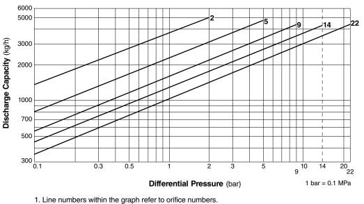
2. Differential pressure is the difference between the inlet and outlet pressure of the trap.
