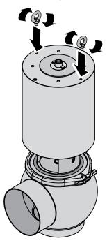
Once valve installation has been completed, remove the eyebolts and put the screws back in.
