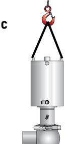
DN125 and DN150 Weight over 50 Kg
