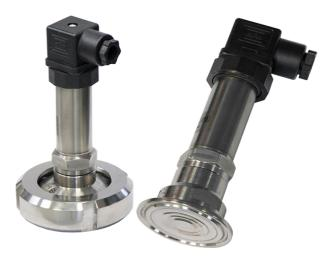
These series of instruments has been designed for pressure transmission. Pressure transmitters detect the pressure of liquid and gaseous fluids by transforming the value into an electrical signal. The sensor used is piezoresistive, consisting of a Wheatstone bridge whose resistances are diffused on a silicon chip. Pressure transmitter with ceramic sensor and calibrated, compensated and amplified signal. They are supplied with current output.
