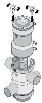
Once valve installation has been completed, remove the eyebolts and put the screws back in
