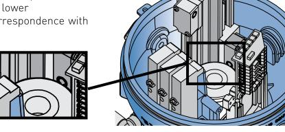
5 Activate the lower lift with regulated air at 6 bar in the upper air connection in the actuator.
