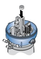
3 Screw the cam on the shaft, spacer will limit the lower lift downward stroke, when seat lift is actuated.
