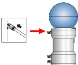
6 If the Proximity switch is correctly calibrated (screw positioning), it must NOT send a feedback signal, and its LED should be OFF. Lower seat is now consider open with the 1.59 mm downward movement offset set by the spacer.
