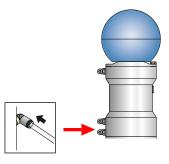
Adjust and regulate the proximity switch position until the lower middle section of the sensitive area is in correspondence with the upper edge of the upper shutter.
